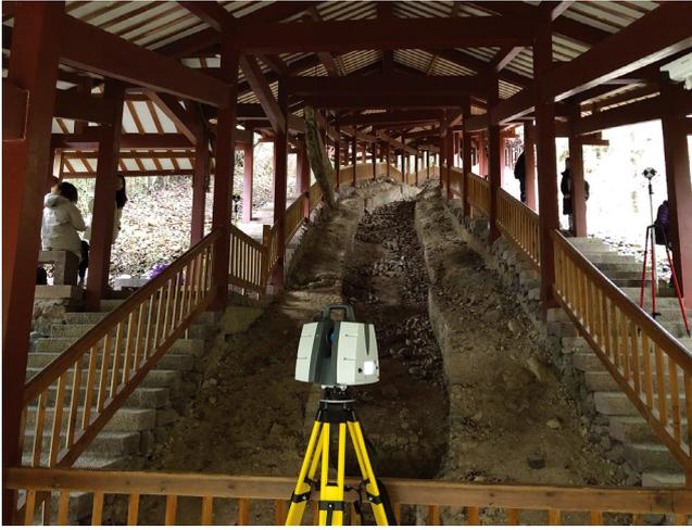
Figure 2: AIM Team uses a 3D scanner to map out the Yulinting kiln site of the Song period in Mt. Wuyi. Here the scanner is placed before the Dragon Kiln to scan from bottom to top.
