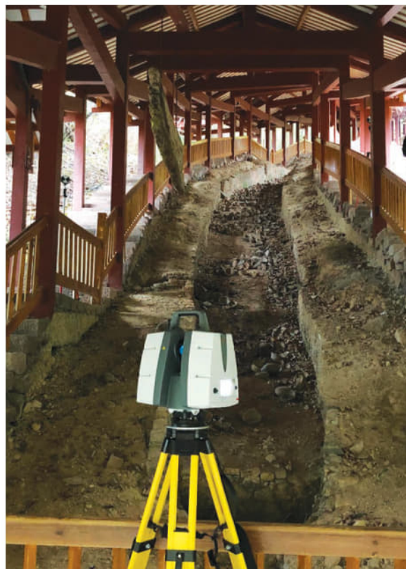
In December 2019, Dr. Li and AIM Team uses a 3D scanner to map out the Yulinting kiln site of the Song period in Mt. Wuyi. Here the scanner is placed before the Dragon Kiln to scan from bottom to top.
